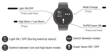
You can turn u8 off, on, and change modes with a remote controller. However, if you manually turn off U8 with the button on the U8 body, you cannot turn it on with the remote controller.
