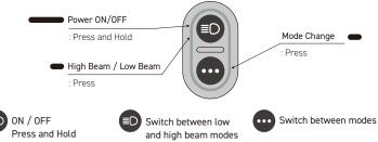
When you start using it on a new day, you need to press the button on the U8 body to turn on the light.
